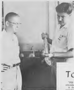
WITNESSING REID test in No. 1 Laboratory is Lt. M. H. Doyle, Navy oil inspector, Tester is J. Ras, checking jet fuel vapor pressure. PRESENCIANDO REID test den Laboratorio No. 1 ta Lt. M. H. Doyle, inspector di azeta di Navy, Tester ta J. Ras, controlando e tension di vapor di jet fuel.
